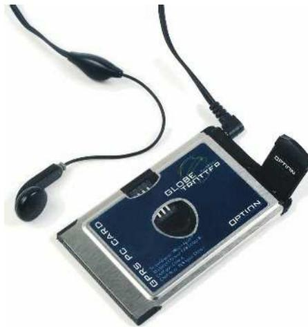
Figure A.2: GlobeTrotter Universal Tri-band GPRS/GSM PC-Radio Card
