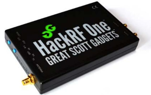
A \$350 HackRF SDR, capable of TX/RX from 10MHz-6GHz
